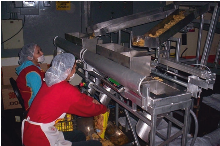
Fig. 7.9 Device for filling of corn tortilla chips
