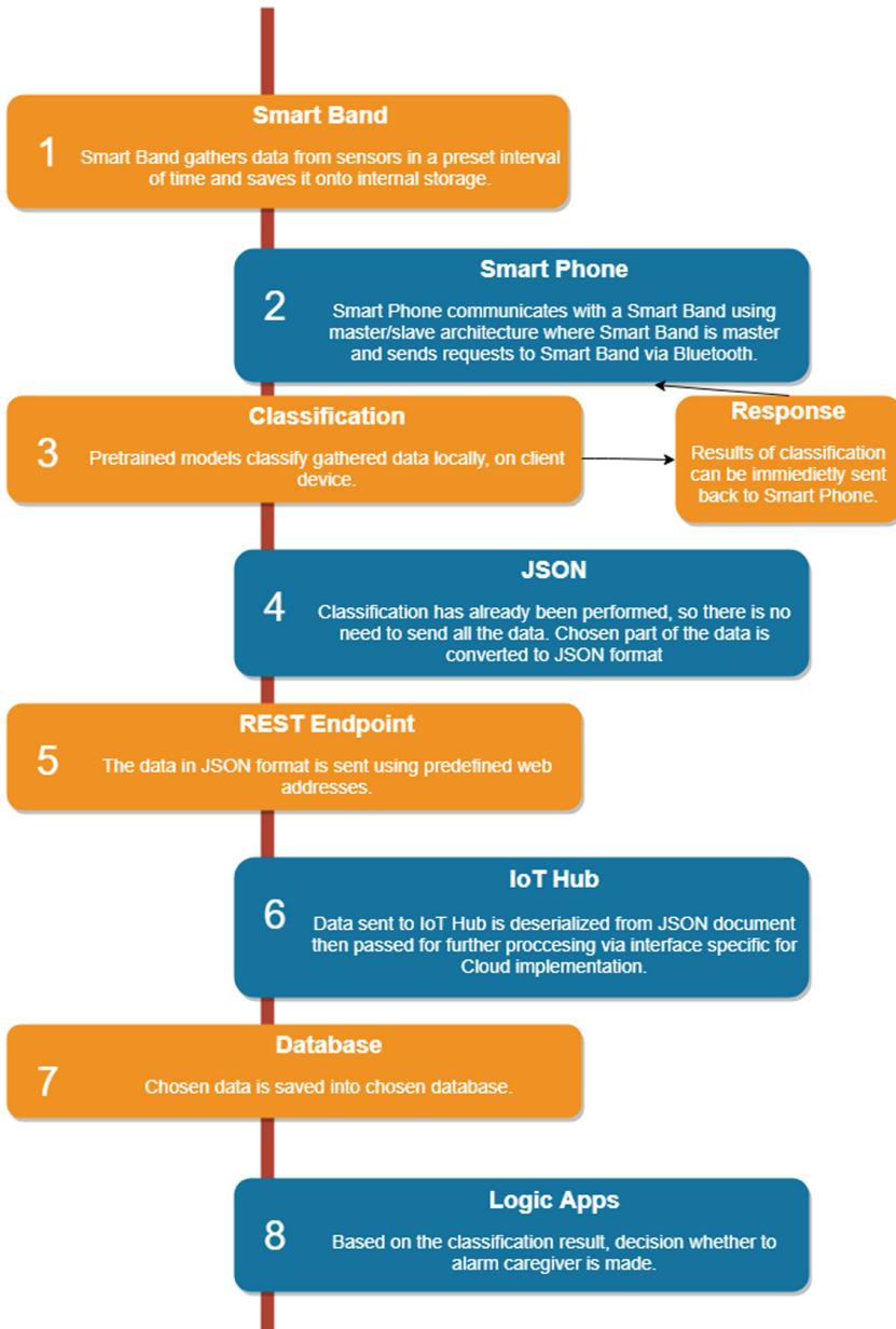
Fig. 3. Communication and flow of data in the system architecture with Edge data processing where classification occurs on the client's device (a smartphone).
