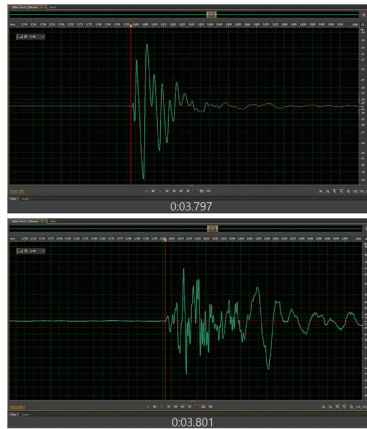
Fig. 22. The moments of wave first-breaks for test 4.9
