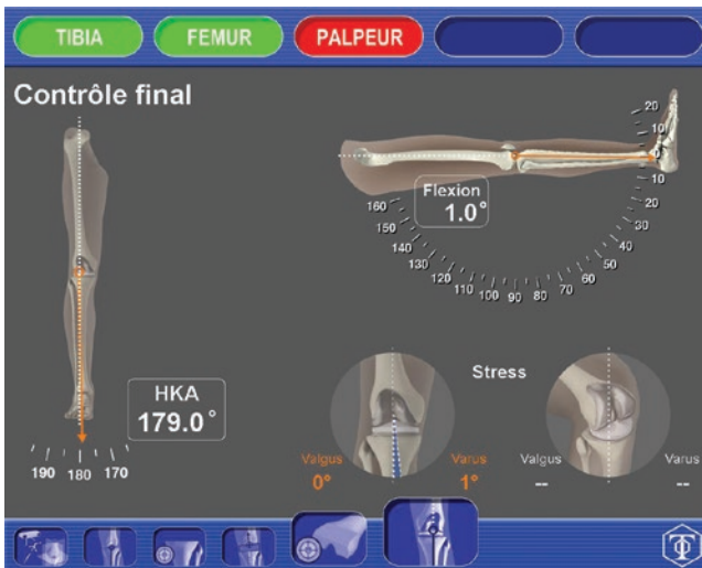
Fig. 28.19 Final check of the HKA angle, laxity in extension/flexion and maximal flexion
