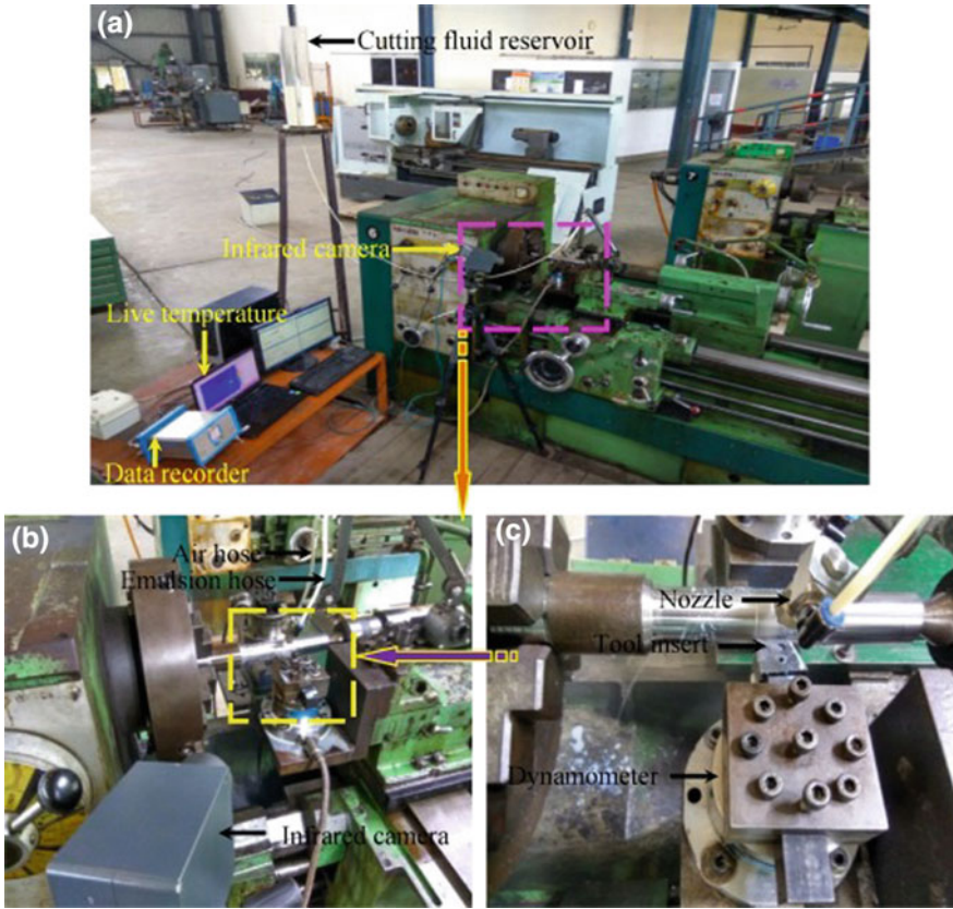
Fig. 11 Minimum quantity cutting fluid experimental setup [60] with kind permission from Elsevier
