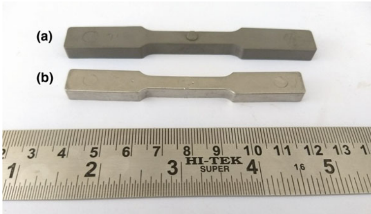
Fig. 13 Comparison of a green and b sintered part
