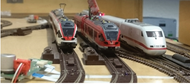
Fig. 6. The physical demonstrator component. Shown are the modified model trains with the Bluetooth-LE (red PCB) back-channel to notify balise detection for odometry. The IRDA balises are seen in the foreground tracks between the white ribbon-cables connected to the IR-PCB. (Color figure online)
