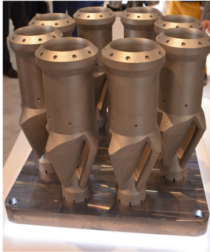
Fig. 3. Elements on the production platform. Not cut off. [own source - FORMNEXT 2018]
