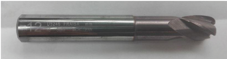
Fig. 6. Corner radius end mill: FRAISA U5246.
