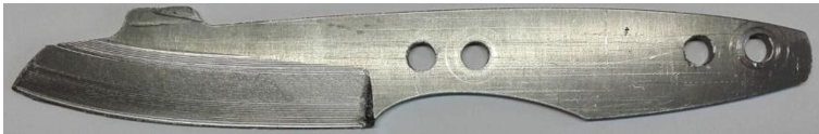
Fig. 24. Knife with main bevel made by morph strategy (ball nose end mill).
