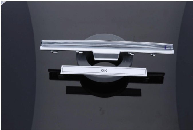
Fig. 4. Product subject to visual assessment after the electroplating process - a strip for a passenger car.
