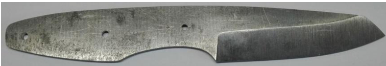
Fig. 28. Knife with main bevel made by grinding.
