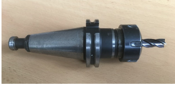
Fig. 4. Short clamp milling tool.
