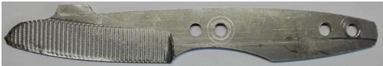
Fig. 19. Knife with main bevel made by parallel strategy variant I.
