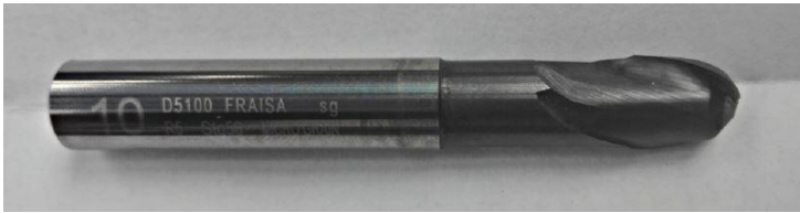
Fig. 5. Ball nose end mill: FRAISA D5100.
