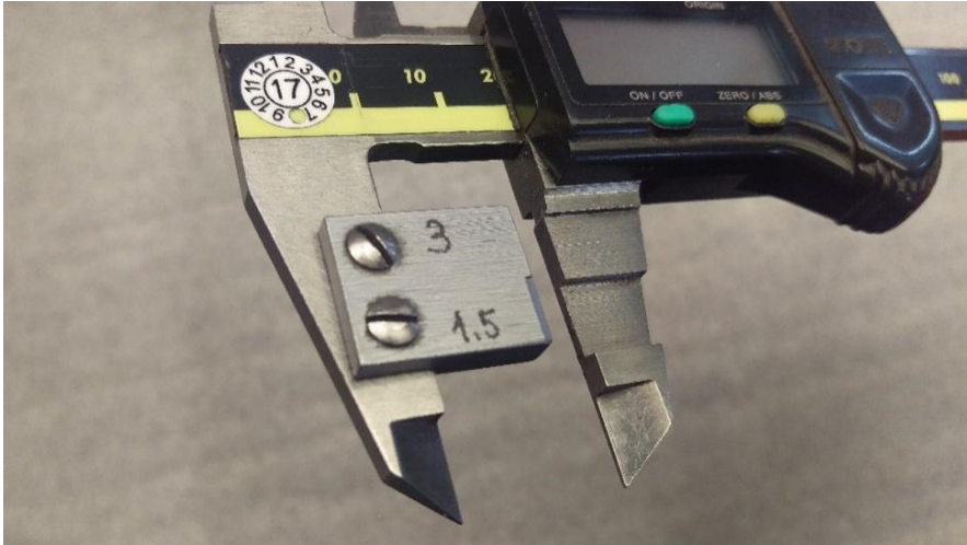
Fig. 1. Electronic caliper with metal plates and visible milling of the jaws (own elaboration).
