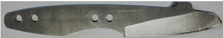
Fig. 21. Knife with main bevel made by parallel strategy (A).
