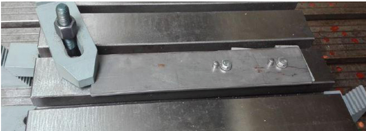
Fig. 10. Mounting the flat bar in the machining fixture.
