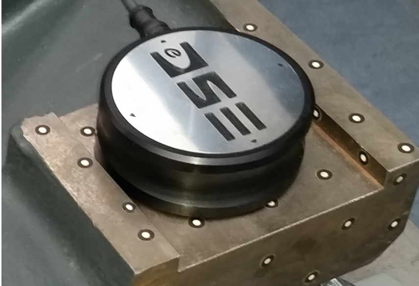
Fig. 2. View of the inclinometer sensor inside a casing which is placed on the workpiece surface.
