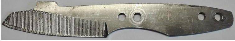
Fig. 20. Knife with main bevel made by parallel strategy variant II.
