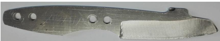
Fig. 22. Knife with main bevel made by parallel strategy (B).
