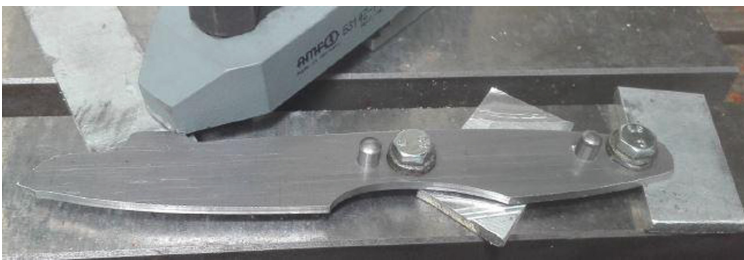
Fig. 11. Mounting the knife after cutting out the shape.
