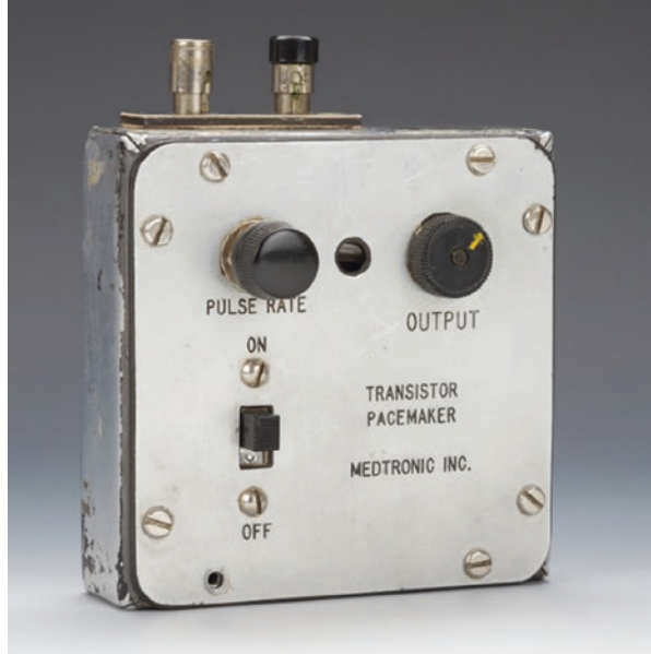
Fig. 9.8 First pacemaker prototype. Source: Historical perspective of cardiovascular devices and techniques associated with the University of Minnesota. In: Iaizzo PA, editor. Handbook of Cardiac Anatomy, Physiology, and Devices, third edition. Springer International Publishing AG, Switzerland, 2015, Fig. 25.13(a)
