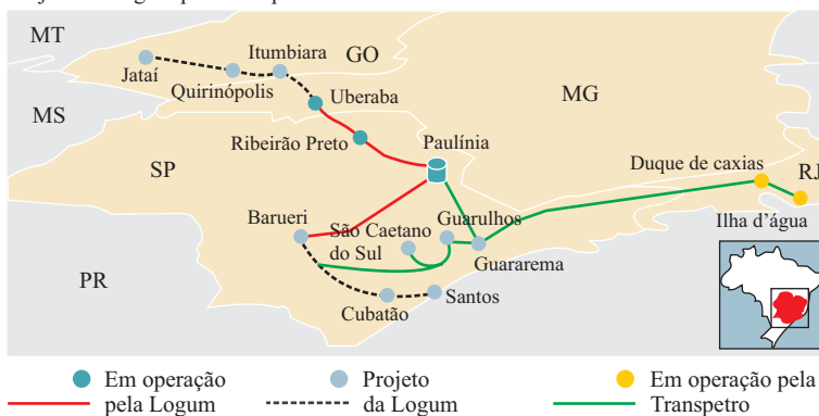
Fig. 18.9 Ethanol transportation through dedicated pipeline in Brazil. (Source: Souza, Z. 2018 (UNICA apud ABAG), personal communication)
