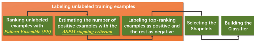
Fig. 2. The workflow of our PU-Shapelets (PUSH) algorithm.
