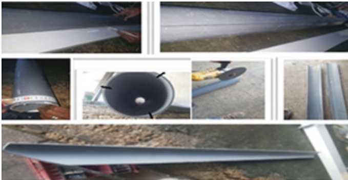
Fig. 29.5 Building steps of the blades out of PVC pipes
