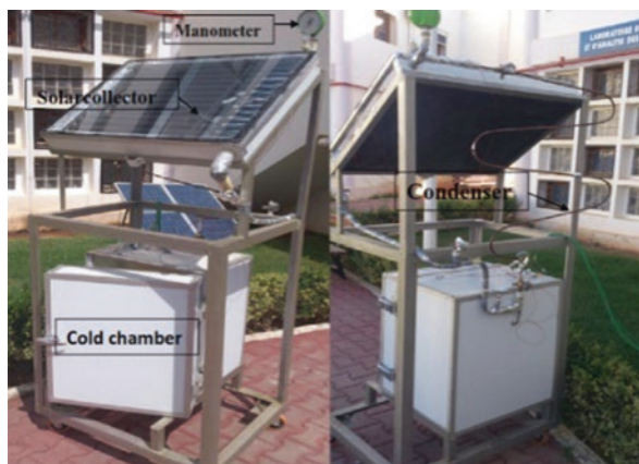
Fig. 78.3 Photograph and plan of adsorptive solar refrigerator [19]
