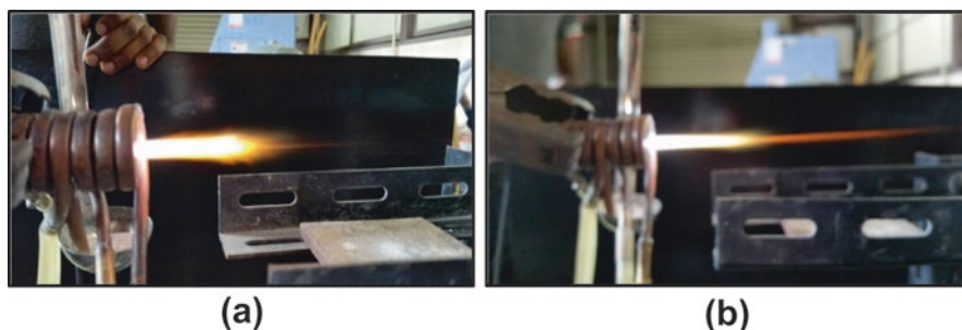
Fig. 79.2 Appearances of the air plasma jets. (a) Air plasma jet. (b) Feedstock injected
