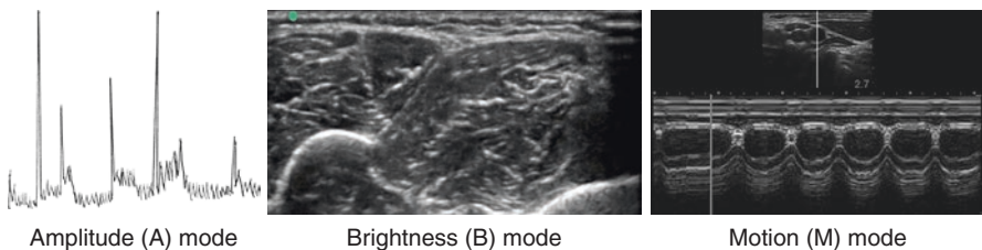
Fig. 1.5 Three different modes of ultrasound. (Reprinted with permission from Philip Peng Educational Series)
