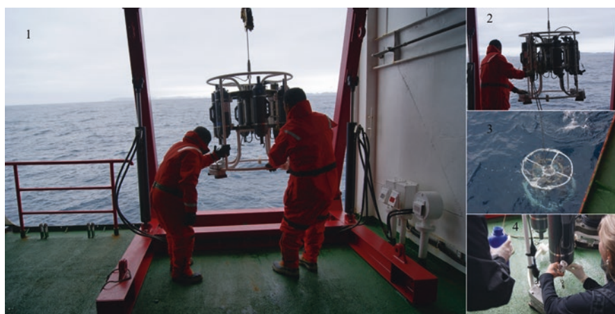
Fig. 10.7 Sequential process of seawater sampling using a combined Sea-Bird CTD equipped with 24 5L Niskin Sampling Bottles. (Photos Credits: LH Rosa)
