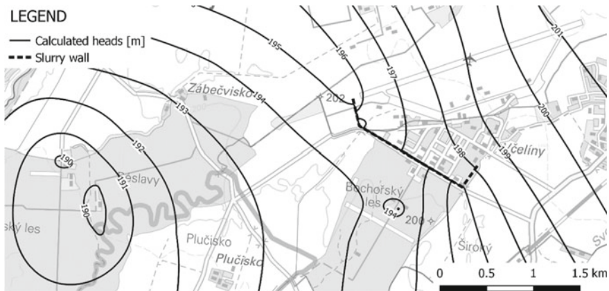
Fig. 8.8 Simulation of the effect of protecting subsurface wall and groundwater pumping in localities Bochoř and Troubky [22]
