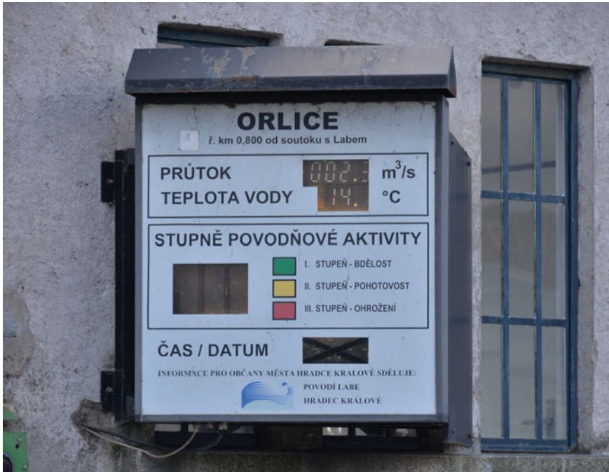
Fig. 15.8 Information for the general public—water flow, temperature of water and level of flood activity. Orlice River in Hradec Králové, 800 m far from confluence with Labe river. Administrator: Labe River Board, s. e. (Photograph: Jiří Schneider)
