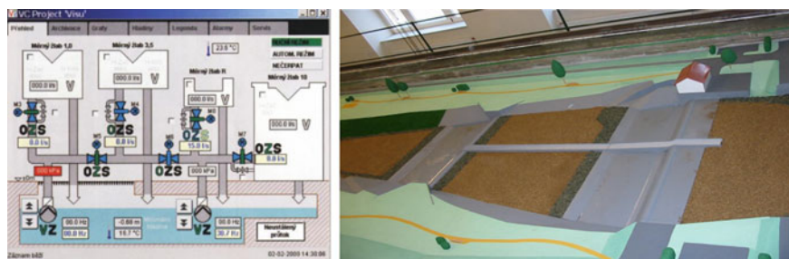
Fig. 2.16 Visualisation of an innovated hydraulic circuit (left), a model of the Hrabovský weir on the River Ostravice with a scenario of a solution of a fish ladder, at a length scale of 1:50 (right)
