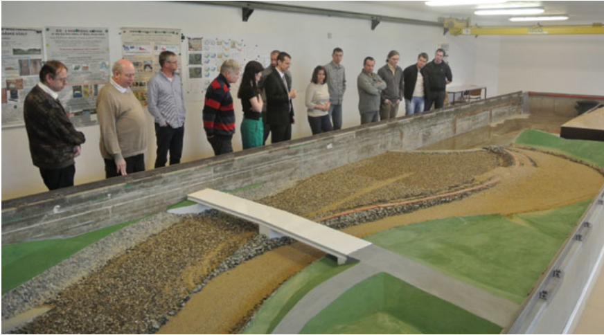
Fig. 2.23 Presentation of the process of sediment transport (a section of the River Opava, at a scale of 1:30) to the representatives of Povodí Odry, s.p. (a state-owned enterprise) and AQUATIS, a.s
