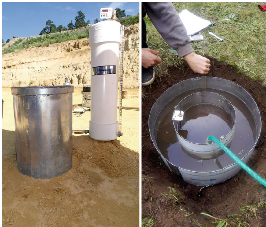
Fig. 4.14 Infiltration test using an infiltration cylinder
