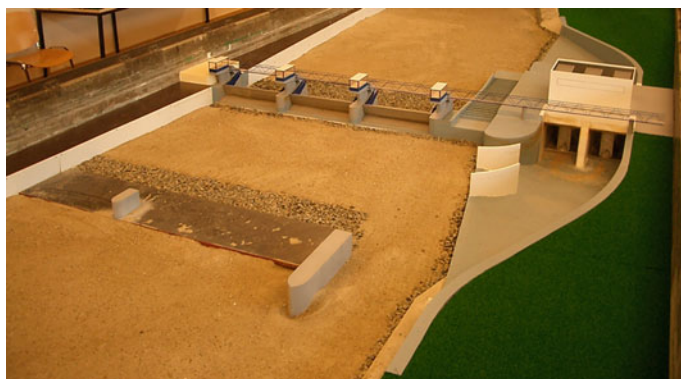
Fig. 15.2 Physical model of the weir SHPP
