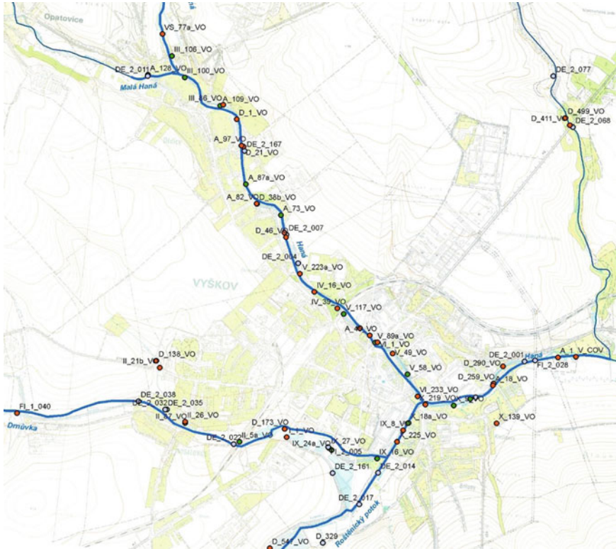
Fig. 5.12 River network in the Vyškov city with marked sewer overflows: red—existing remaining, blue—existing, blank—proposed
