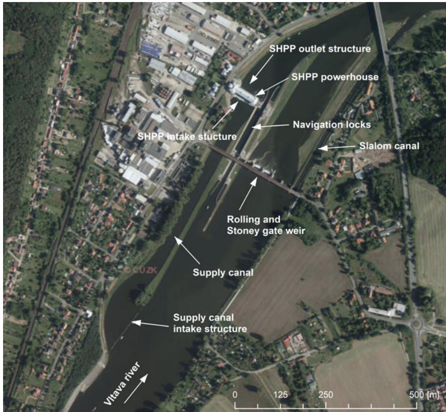
Fig. 15.11 Situation of SHPP Miřejovice (based on data [10])
