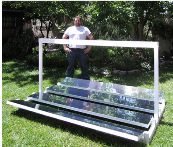
Fig. 19.11 Compact Fresnel collector
