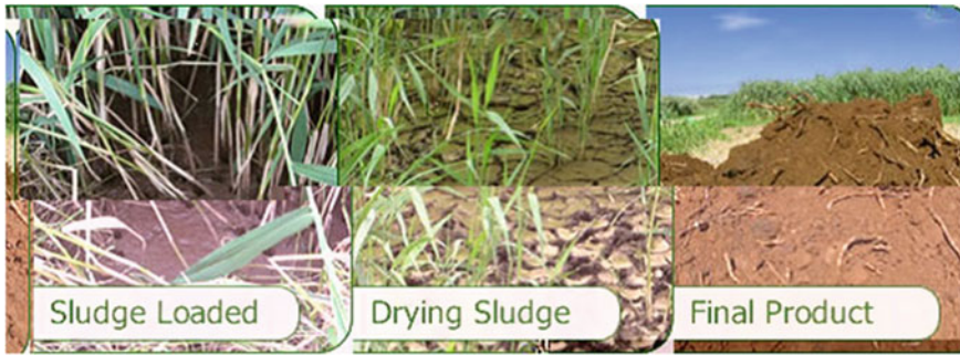
Fig. 15.7 Example of sludge loading, drying, and the final product
