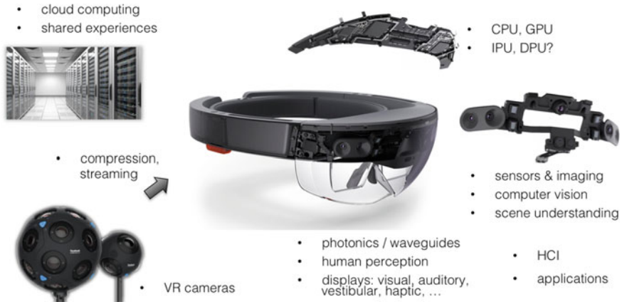
Fig. 25.1 Overview of components of AR/VR systems. From dedicated, application-specific processors to microdisplays, photonic waveguides, 360° cameras, novel cloud services to new approaches to computer vision and human-computer interaction, AR/VR system design includes a plethora of aspects that all together define the user experience. Parts of this image are reproduced from Microsoft and Facebook promotional material
