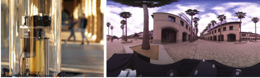
Fig. 25.8 SpinVR: a rotating camera with two line sensors directly captures omnidirectional stereo panoramas
