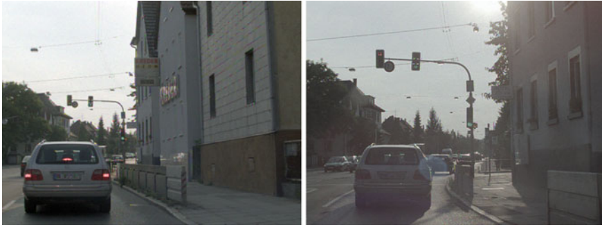
Fig. 21.8 Two images of a video sequence taken with the HDRC sensor of a road scene demonstrating the need for high dynamic range acquisition with direct sun in view (right)
