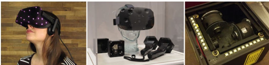
Fig. 25.7 Examples of optical tracking in VR. Left: near-infrared (NIR) LEDs of the Oculus Rift recorded with a camera that is sensitive to NIR (image reproduced from ifixit.com ). Center: HTC Vive headset and controllers with exposed photodiodes (image reproduced from roadtovr.com ). Right: disassembled HTC Lighthouse base station showing two rotating drums that create horizontal and vertical laser sweeps as well as several LEDs that emit the sync pulse (image reproduced from roadtovr.com )
