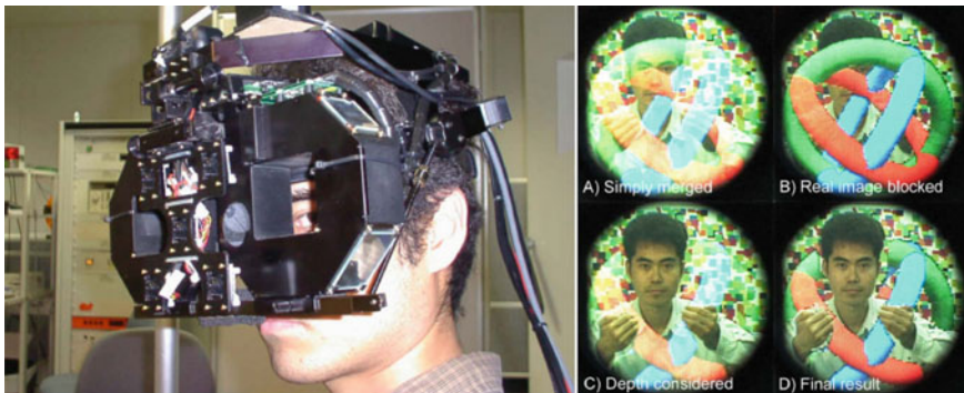
Fig. 25.6 Occlusion-capable optical see-through AR display (left). The display includes relay optics and spatial light modulators that allow for hard-edge per-pixel control of the observed scene before it hits the user’s retina. The right panel shows views through the display with a no occlusion control, i.e. digital and physical image are simply superimposed, b occlusion enabled to block light from the physical scene everywhere where there is digital content, c occlusion disabled but depth considered, i.e. physical objects can occlude digital objects but selectively rendering the latter, d occlusion enabled and depth considered, i.e. both physical and digital objects can correctly occlude the other one. Figure reproduced from [90] © IEEE 2003
