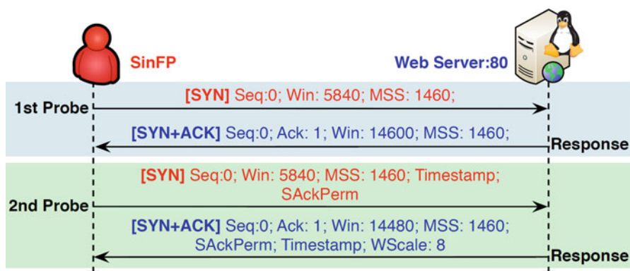
Fig. 8 Packets exchanged during a SinFP scan
