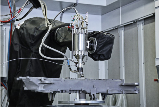
Fig. 7. Cold spray developed by GE Avio. Source: https://www.ge.com/reports/secret-weapon-supersonic-blaster-rebuilds-jet-parts-flying-powder/ [47]
