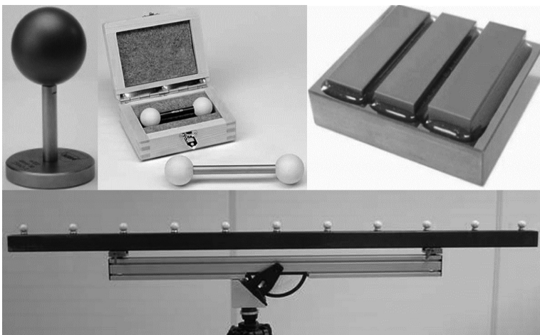
Fig. 1. Existing artefacts for testing optical CMMs [11, 13]
