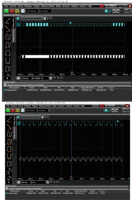
Fig. 4. Optical signal square wave of 3.76 MHz (left) and 20 MHz (right).
