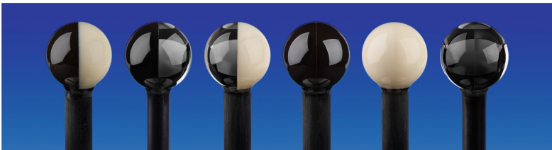
Fig. 10. Set of multi- and mono-material spheres used for the assessment of the P -test. From left to right: three MuMat-spheres \text{Al}_2\text{O}_3 & \text{Si}_3\text{N}_4 , \text{Si}_3\text{N}_4 & N-SF6 and \text{Al}_2\text{O}_3 & N-SF6; and three MoMat-spheres \text{Si}_3\text{N}_4 & \text{Si}_3\text{N}_4 , \text{Al}_2\text{O}_3 & \text{Al}_2\text{O}_3 and N-SF6 & N-SF6.
