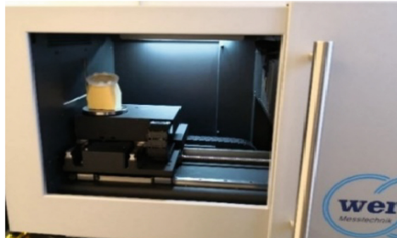
Fig. 4. Measurement of 3D printed component with CT [17]
