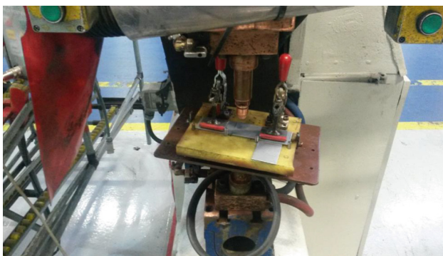
Fig. 6. Fixture apparatus for spot welding of testing specimens
