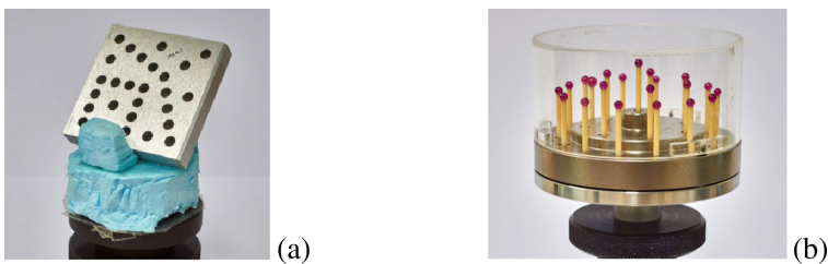
Fig. 3. Example of length reference standards (source: [5]) (a) PTB aluminium hole plate; (b) multi-sphere standard.
