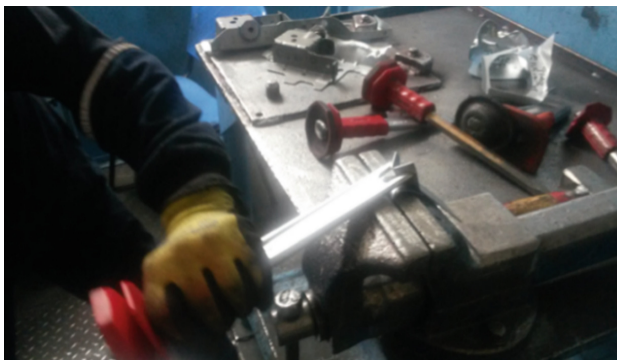
Fig. 5. Application of the destructive testing for specimens to determine welding parameter limit values
