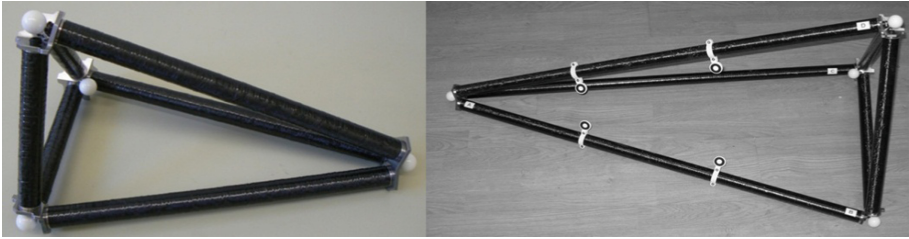
Fig. 3. Small (left-hand picture) and large tetrahedron artefacts [11]
