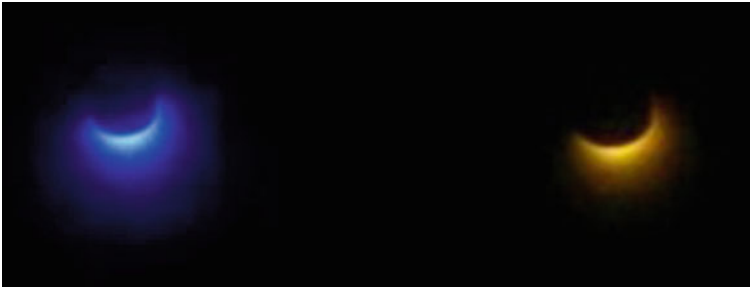
Fig. 6 Comparison between a white (on the left) and a yellow (on the right) card illuminated using a blue laser
