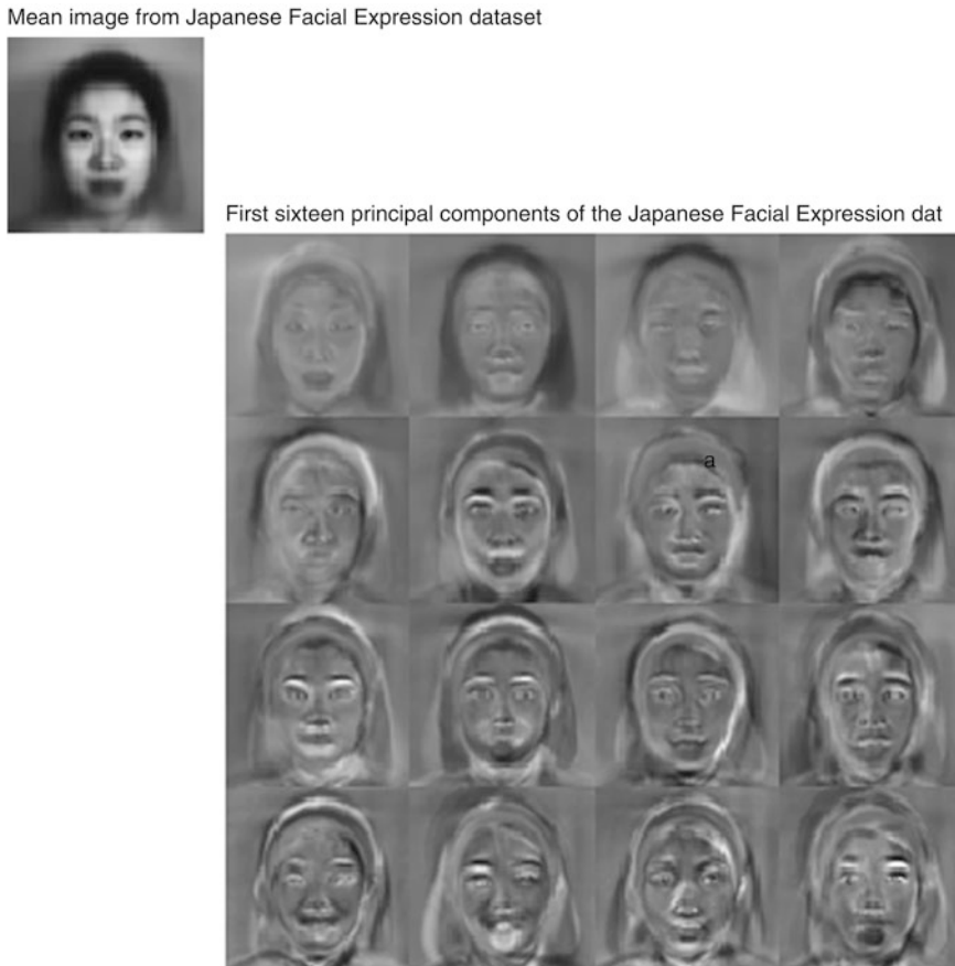
Figure 5.10: The mean and first 16 principal components of the Japanese facial expression dataset
