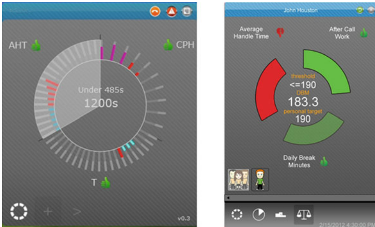
Fig. 3 The original design for the data visualization widget can be seen on the left. The simplified version based on feedback from the business group can be seen on the right
