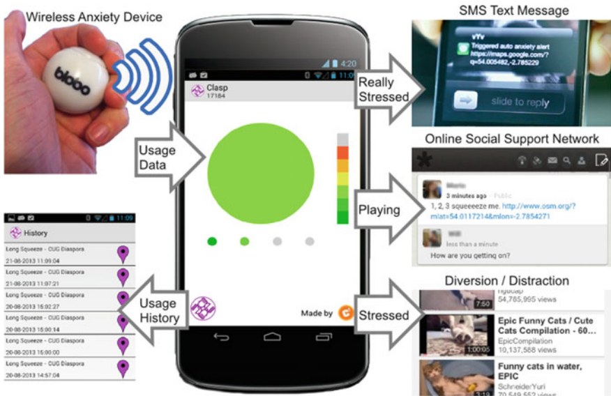
Fig. 2 Clasp: A digital tactile anxiety management device supporting self-reflection
