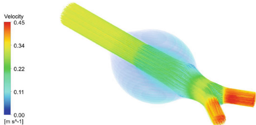
Fig. 13 Representation of the velocity streamlines for the model of the abdominal aorta with aneurysm and short stent graft
