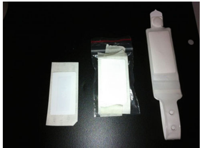
Fig. 7 RFID tags used as internal tag, drug tag and patient tag
