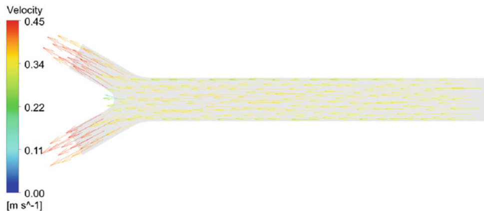
Fig. 5 Velocity vector distribution for the model of the healthy abdominal aorta
