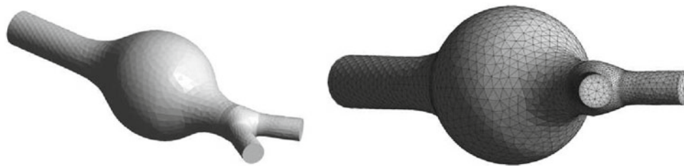
Fig. 2 Geometry (left) and computational mesh (right) of the numerical model of abdominal aorta
