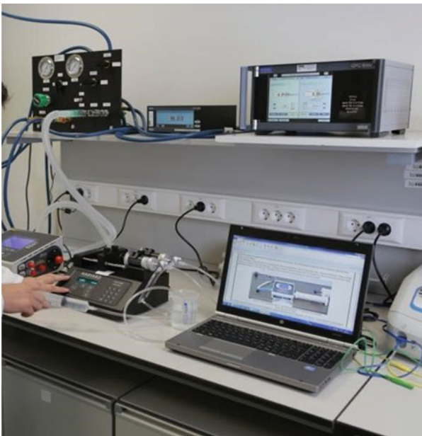
Fig. 2 Calibration systems for simulators and analyzers at TÜBİTAK UME Medical Metrology Research Laboratory
