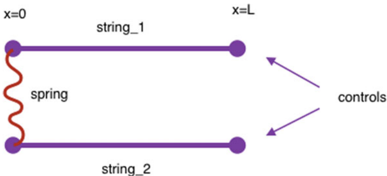
Fig. 1 Two strings coupled via an elastic spring and masses
