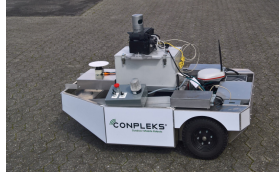
Fig. 3. Compleks' robot created for collecting golf balls autonomously [32].
