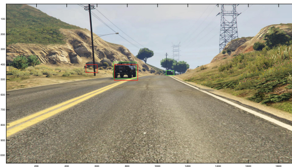
Fig. 4. GTA frame with red bounding boxes around cars detected by YOLO, and green boxes around true cars. Note the red box around the bush on the left, indicating a YOLO false positive, and the lack of red box around the faraway car on the right, indicating a YOLO false negative. The red box in the middle is a true positive. (Color figure online)
