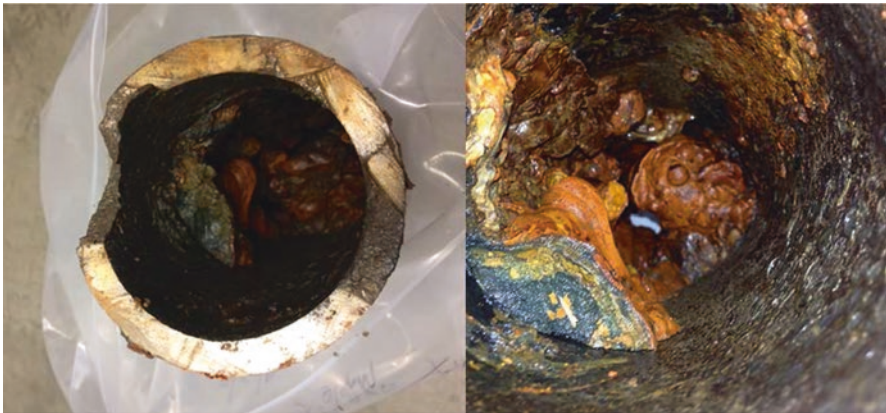
Fig. 8.3 Left photo shows the cross section of a 4-inch cast iron pipe taken off service from the Fayetteville DWDS (AR); right photo shows the close-up shot of biofilms formed within the same pipe
