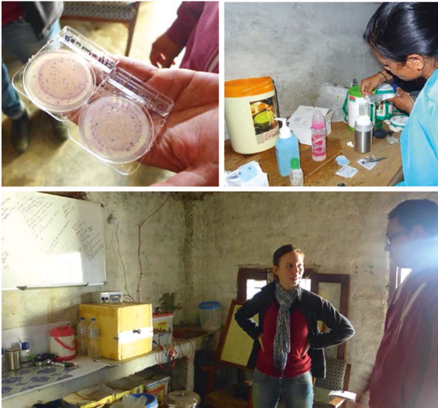
Fig. 3.4 Photos of field equipment for microbial water quality testing in Nepal. (Photo credit: Dorian Tosi Robinson and Sara Marks)
