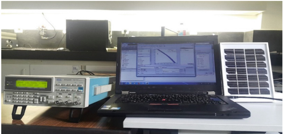
Fig. 6. Signal generator and DAQ connects with workstation.
