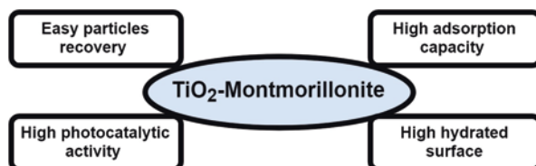
Fig. 13.7 Main advantages of \text{TiO}_2 -Montmorillonite-based composites compared to \text{TiO}_2
