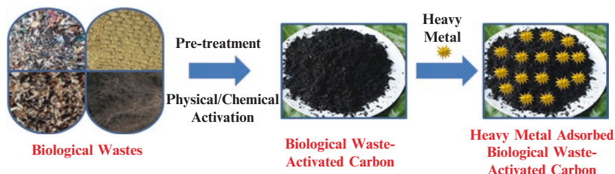
Fig. 3.2 Synthesis of activated carbon from biological waste materials for heavy metal removal
