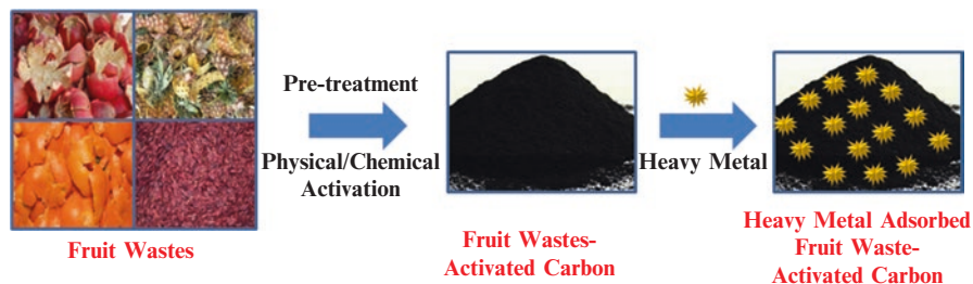
Fig. 3.3 Synthesis of activated carbon from fruit waste materials for heavy metal removal
