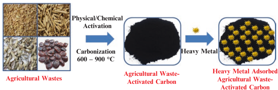
Fig. 3.1 Synthesis of activated carbon from agricultural waste materials for heavy metal removal
