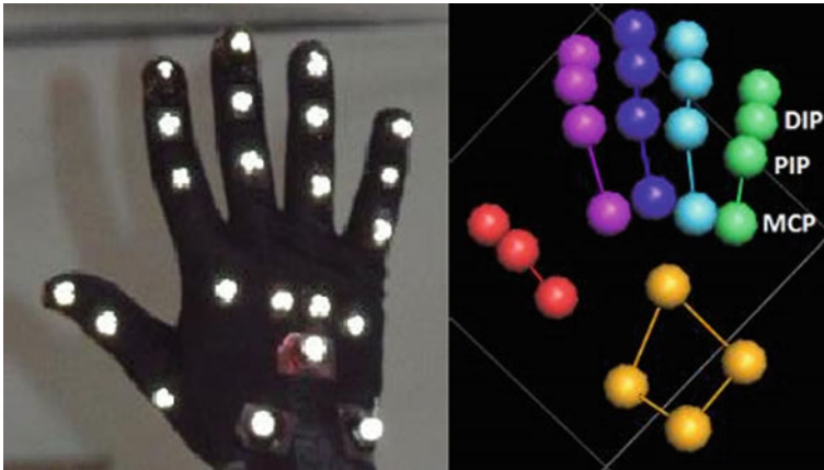
Fig. 1.2 Position of the markers on the hand
