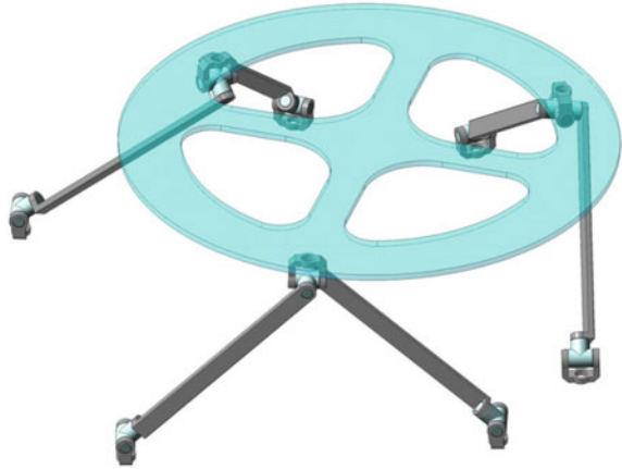
Fig. 5.3 Structural group with parallel chains having zero DoF
