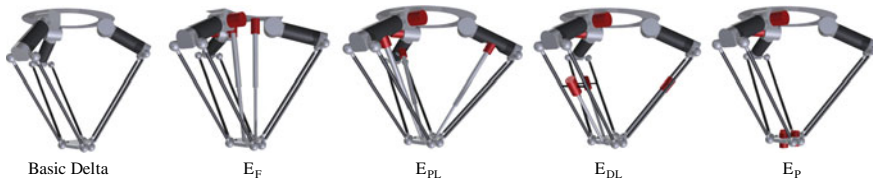
Fig. 11.1 Illustrations of translational 3-dof Delta robot and 6-dof variants with functional extensions
