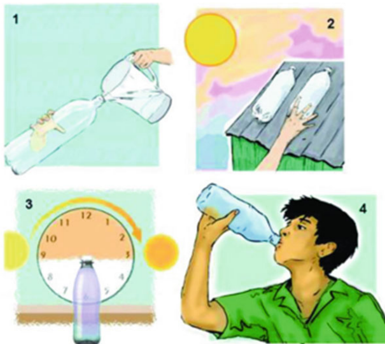
Fig. 1.6 A simple household-based water purification system for solar disinfection of water SODIS process. (McGuigan et al. 2012)
