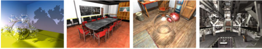
Fig. 7.11 Real-time renderings on the RPU prototype using a single FPGA running at 66 MHz and 512 \times 384 resolution: SPD Balls (1.2 fps, with shadows and refractions), a conference room (5.5 fps, without shadows), reflective and refractive spheres-RT in an office (4.5 fps), and UT2003 a scene from a current computer game (7.5 fps, precomputed illumination)
