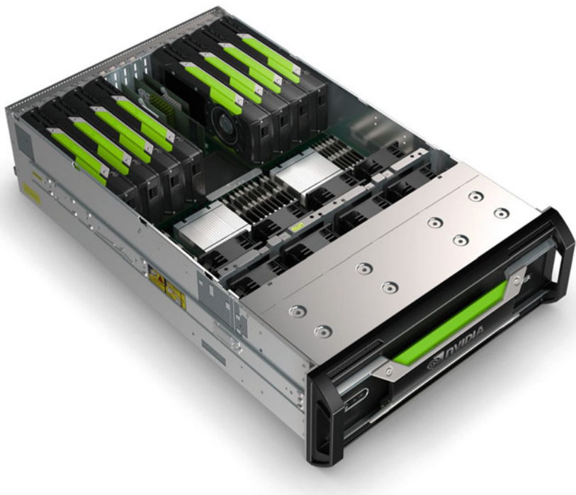
Fig. 7.13 Physically based rendering for the whole team: Nvidia’s 56 TFLOPS (and $50,000) Quadro VCA. Source Nvidia
