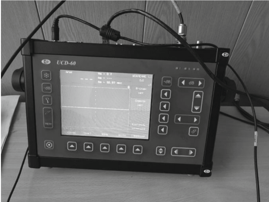
Fig. 1 Industrial ultrasonic flow detector USD60-N
