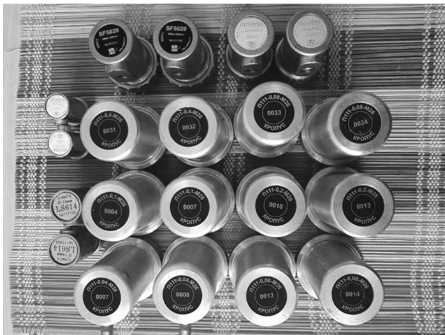
Fig. 2 A set of low-frequency ultrasonic sensors used in the measurements
