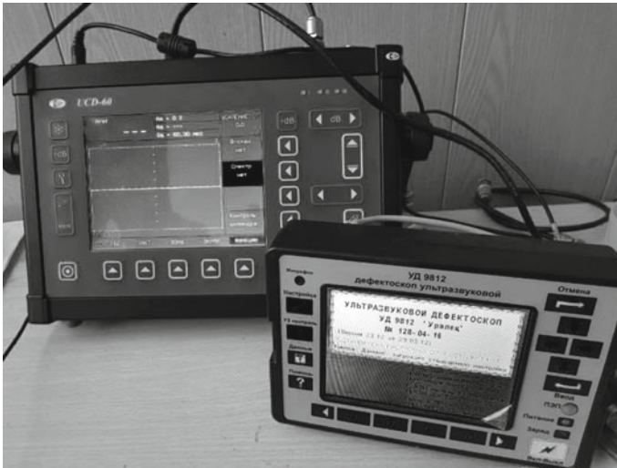
Fig. 2 Flaw detectors used for measurements. Left—low-frequency flaw detector USD60-N, right—UD9812
