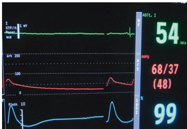
Fig. 30.3 Electrocardiography, invasive arterial blood pressure and pulse oximetry monitoring showing asystole episode due to surgical retraction near the cerebellopontine angle
