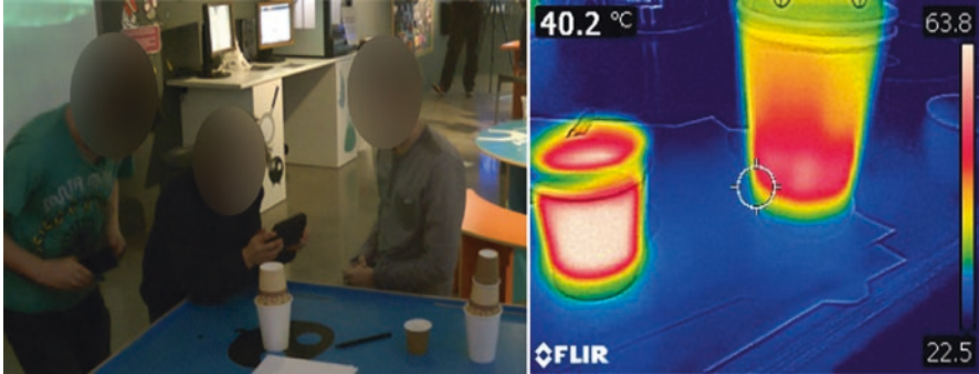
Fig. 1 Three peers observing the efficiency of their modelled paper cup thermoses using a thermal camera. The pupil in the centre directs the camera towards the thermoses (left). A corresponding thermal image viewed on the camera display and captured by the group during the activity (right)
