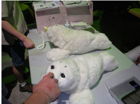
Fig. 5.2 Care Robot Paro, it is touch sensitive and interacts with users while being fondled Source CC-BY-SA-2.0 (Biggs 2005)
