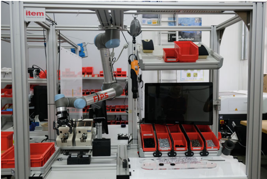
Fig. 6.2 Assembly cell with the UR-5 hanging from the ceiling
