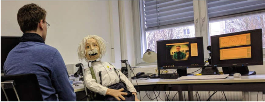
Fig. 5.1 Cameras in the eye of the robot detect pulse rate and heart rate variability in order to enable natural communication between the social robot and the human
