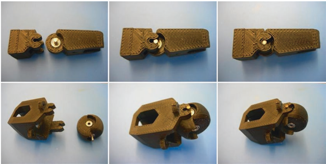
Fig. 21.9 Two examples of assembling a Snap-On joint. Top row: assembling a DIP hinge joint. Bottom row: assembling a MCP ROM-ball on to the finger base
