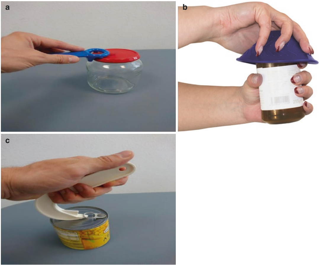
Fig. 19.2 (a) Releasing the vacuum, (b) unscrewing the lid, and (c) opening a tin. (Published with kind permission of © R. Zumhasch 2017. All rights reserved)
