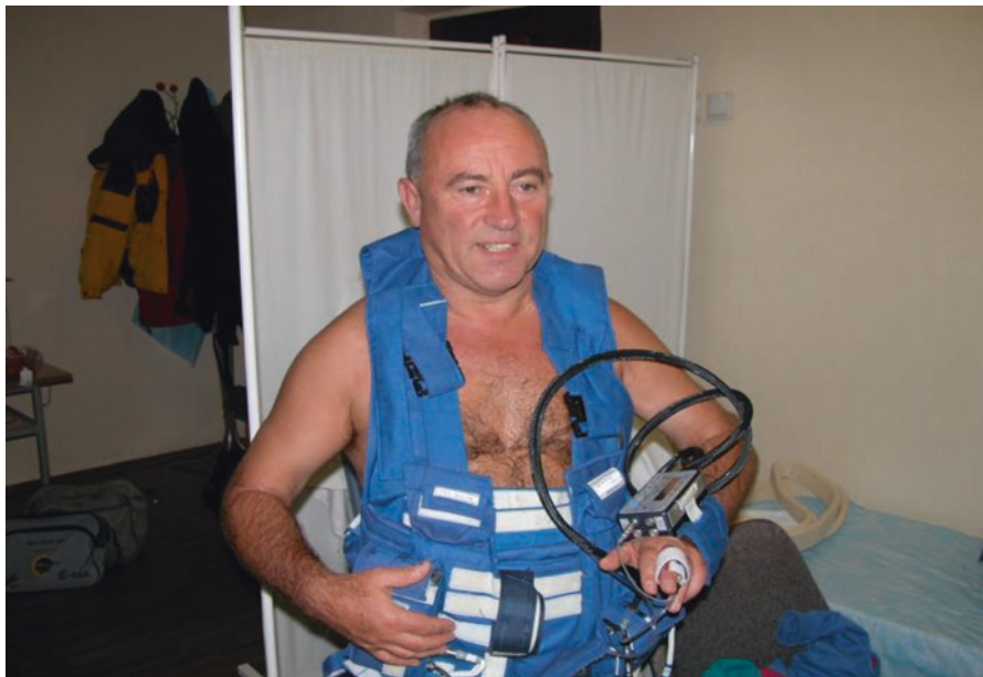
Fig. 23.2 Implementation of measurement device (ECG, finger blood pressure cuff, and respiration detector) and used in the ISS in the period 2000–2011. The system supplied several hundred hours of laboratory-quality recordings on successive astronauts and cosmonauts
