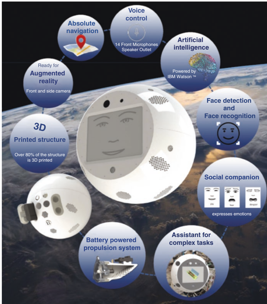
Fig. 21.3 Design concept of CIMON and technical features: The CIMON systems consists of a 3D printed hardware with a battery-powered propulsion system and a variety of intelligent functions such as navigation guidance and control, voice control, and face detection and recognition. Over the time-course of development more features and functions will become available (Source: DLR)
