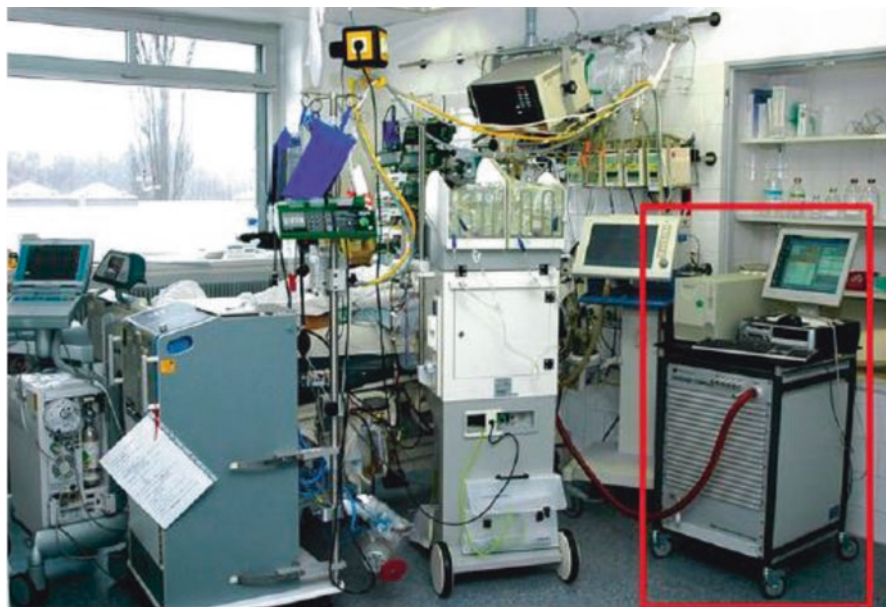
Fig. 24.1 Ion molecule reaction mass spectrometer (IMR-MS, red box ) during online monitoring of exhaled breath in a patient with acute respiratory distress syndrome (ARDS). A directly to the patients endotracheal tube connected steel T-piece allows gas transfer from the patient to the IMR-MS ( red rubber tubing ). The vacuum pumps define the size of the hardware. In space, technical solutions might use the external vacuum instead
