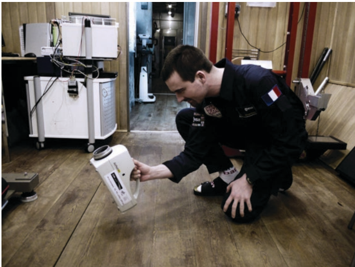
Fig. 37.5 Mars500 crewmember Romain Charles taking an air sample for the microbial experiments (© ESA)
