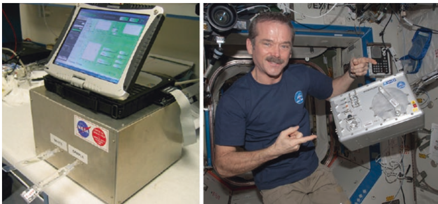
Fig. 27.7 NASA-JSC prototype flight cytometer with sample delivery WBSD units affixed to the sample delivery ports (left); and the Canadian Space Agencies “Microflow” demonstration unit onboard ISS (right)
