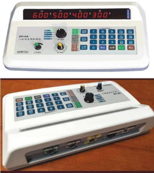
Fig. 20.2 Cardiac electric stimulator can generate programmed stimulation or burst pacing; Its output can be adjusted from 0 to 50 V and pulse width 0–10 ms
