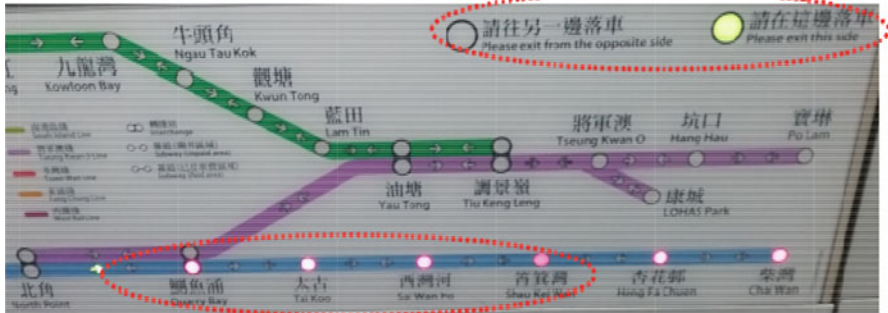
Fig. 9 Example of application of LED display circuits: the route map panel with LED indicators showing the metro stations
