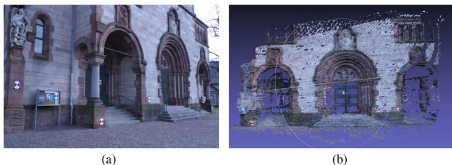
Fig. 8 (a) Original 2D image, (b) dense 3D point cloud estimated with D-ADMM BA (mean re-projection error = 0.76)
