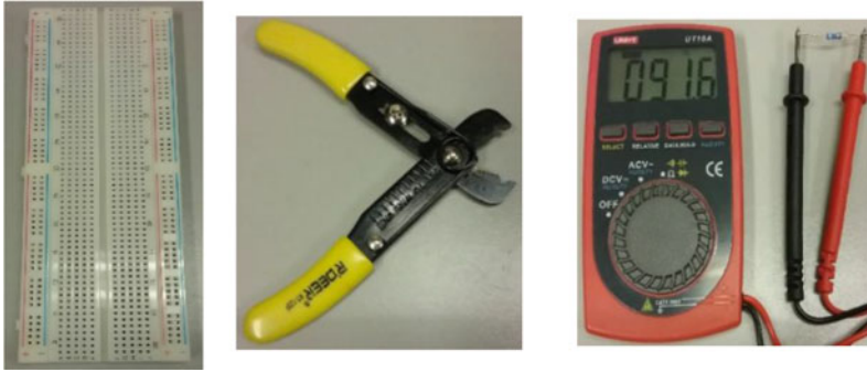
Fig. 4 Very basic tools required for electronic circuit construction: (left) a breadboard, (middle) a wire stripper, and (right) a digital multimeter
