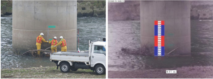
Fig. 6 Japan—River in Niigata: Left: Benchmarks are installed on the wall before testing the system. Middle and right: Water level at different times and the visual imaginary gauge displayed by GUI
