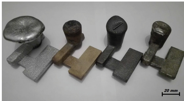
Fig. 3. Demoulded and cleaned castings; from the left: 5A - AlSi 11 alloy, 5B - CuSn10P alloy, 5C - GJL 250 cast iron, 5D - X 5 Cr Ni 18-10 cast steel.
