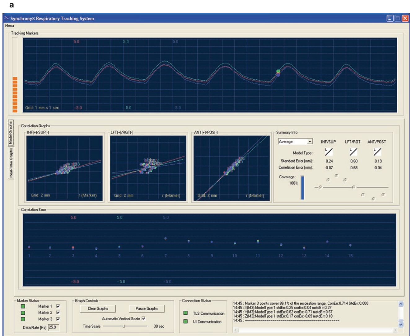
Fig. 3 A Synchrony® (Accuray, Sunnyvale, CA, USA) tracking screen for management of respiratory motion. The respiratory cycle trace from externally placed light-emitting diode (LED) (a) is correlated with the position of fiducials internally implanted into the tumor (the correlation
