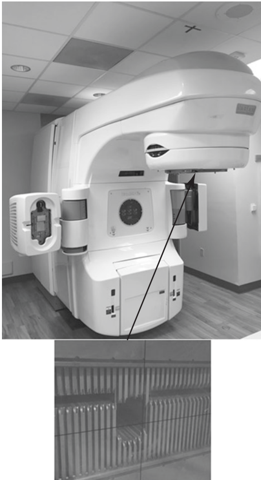
Fig. 5 These images show a modern linear accelerator. Attached to the head of the machine is the micromultileaf collimator, seen in cross section below (follow arrow). The leaves are computer driven to match the shape of the target as the gantry rotates
