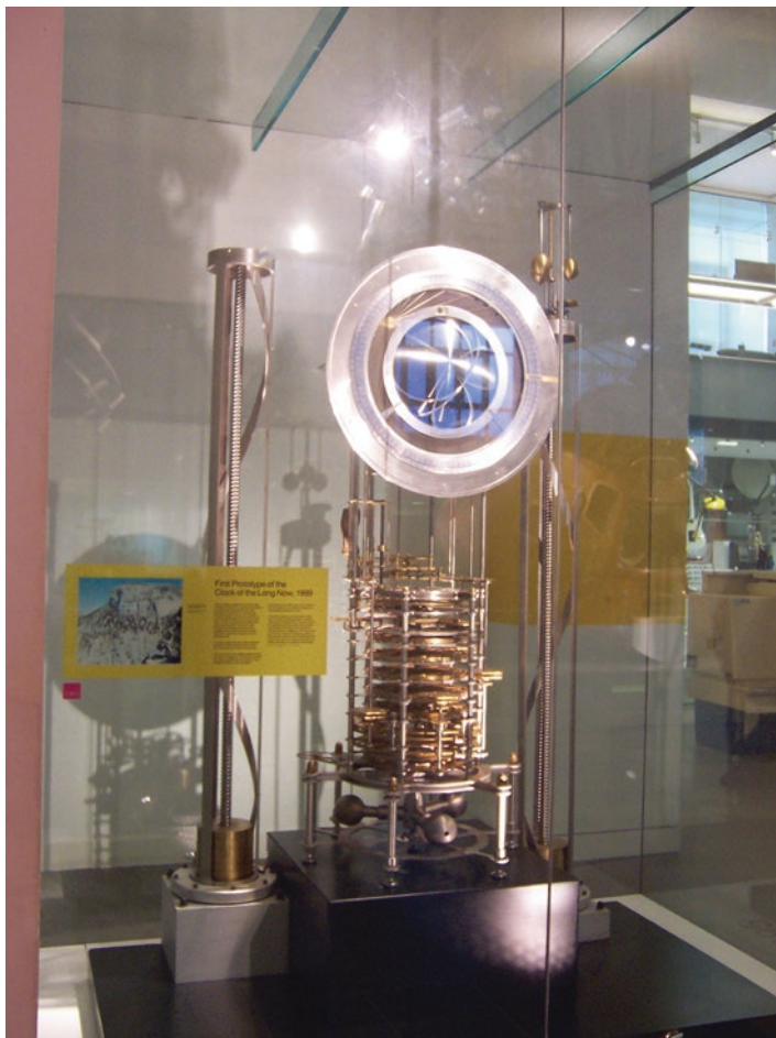
Fig. 16.5 First prototype of the 10,000 Year Clock (1999) on display at the Science Museum in London. The clock ticks once a year. (Courtesy of Pkirlin on en.wikipedia.org )
