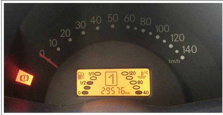
Fig. 4. Attack on the transmission display. The engine was not running but the indicator showed gear 1. The control lights were switched off and the fuel level was increased.
